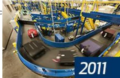
The first of two inline baggage systems becomes operational in November, accelerating the passenger check-in process and enhancing baggage screening capabilities by the Transportation Security Administration. The new automated system relocates the massive luggage scanning process from in front of the ticket counters to an area behind the scenes, reducing congestion in the ticket lobby.
